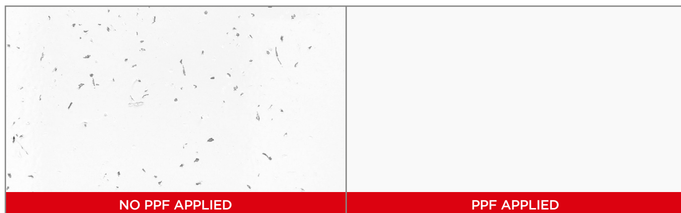
Image represents gravel impact testing on surface with and without PPF installed.
